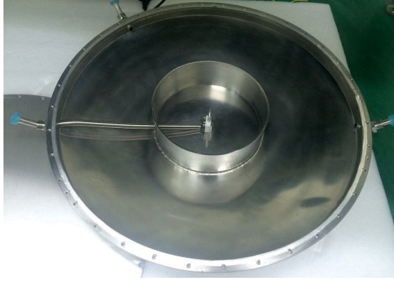
Figure 3.10: The internal structure of the overflow chamber. A level meter in the middle of the chamber. The tube on the left is for liquid xenon out. The other two are for pressure equalizing and overflow-in.
