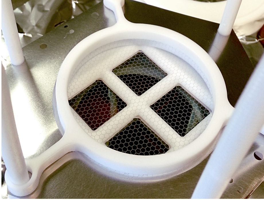
Figure 4.1.6: A photograph of the chemically etched mesh used for all electrodes in the MiX TPC (anode shown). The 50\text{ }\mu\text{m} -thick mesh has a central 76 mm circular region with hexagonally packed grid structure. The hexagons are created at a 2 mm pitch with 50\text{ }\mu\text{m} diameter wires to allow for homogenous TPC field generation while maintaining 95% optical transparency.
