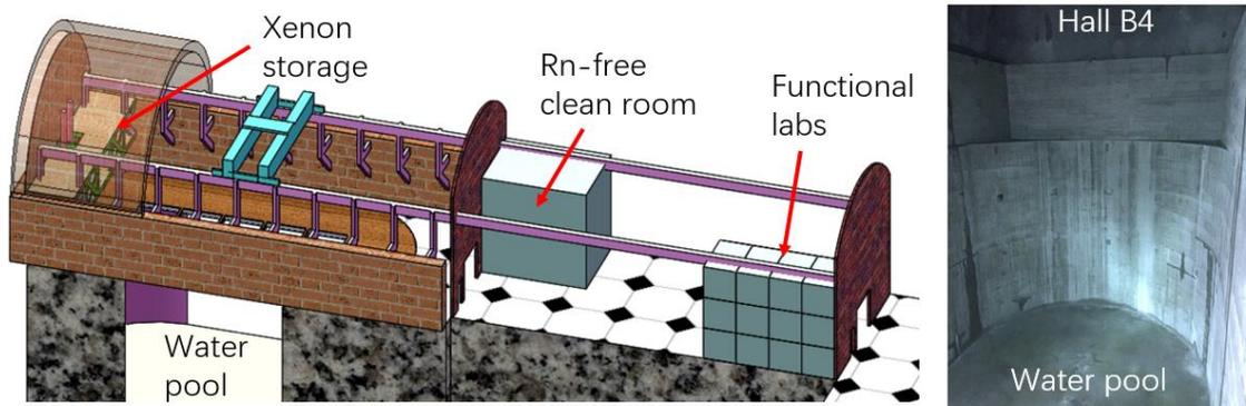
Figure 2: schematic design of Hall B2 in CJPL-II (left), and a picture showing the water pool (right).
